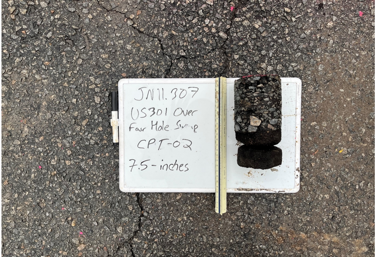
Photograph 6: Asphalt Core CPT-02
