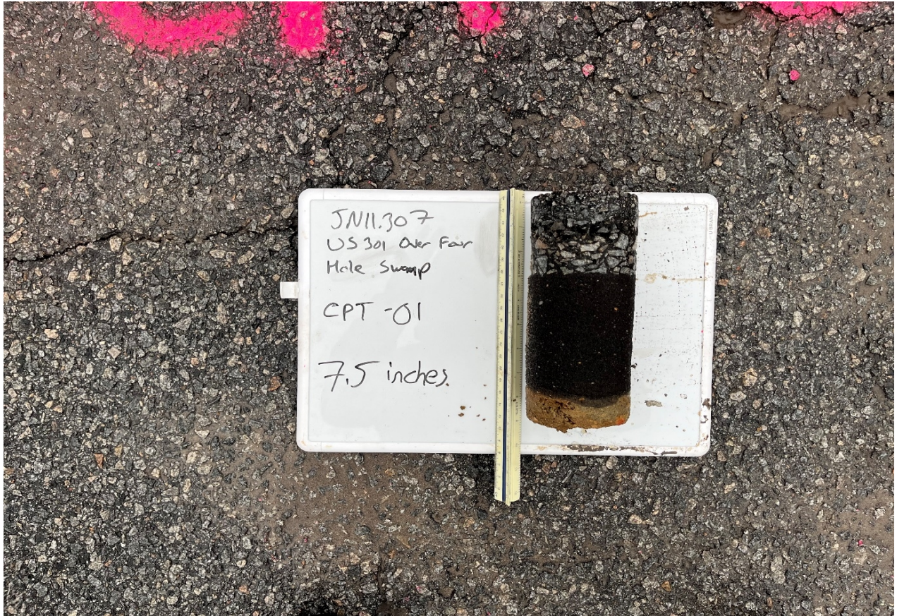
Photograph 5: Asphalt Core CPT-01
